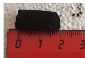
Образец 6, t_{cr}=60\text{ }^{\circ}\text{C} , 950 °C
